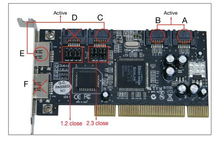
Note: There are six SATA ports in Serial ATA 4-Channel RAID adapter. We named these ports character A through F. Ports A to D are internal SATA ports and E & F are external SATA ports. By changing the jumper setting on the Serial ATA 4-Channel RAID adapter that allows you to utilize 4 ports of this card at the same time. Please set which port to work by jumper setting. By default, Port A, B, C and D are working.
